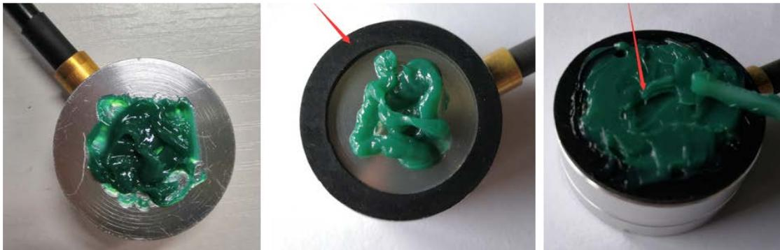
2) Insert the sensor into the holder and install the cover plate
